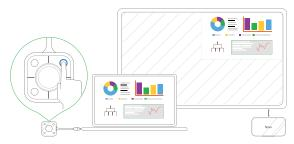
(8) Press any corner button on the LauncherPlus to project your computer's screen onto the corresponding quadrant of the display, the button's blue LED will light when it is in use.
