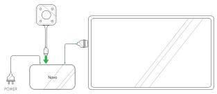
① Connect the LauncherPlus to the NovoConnect device.
